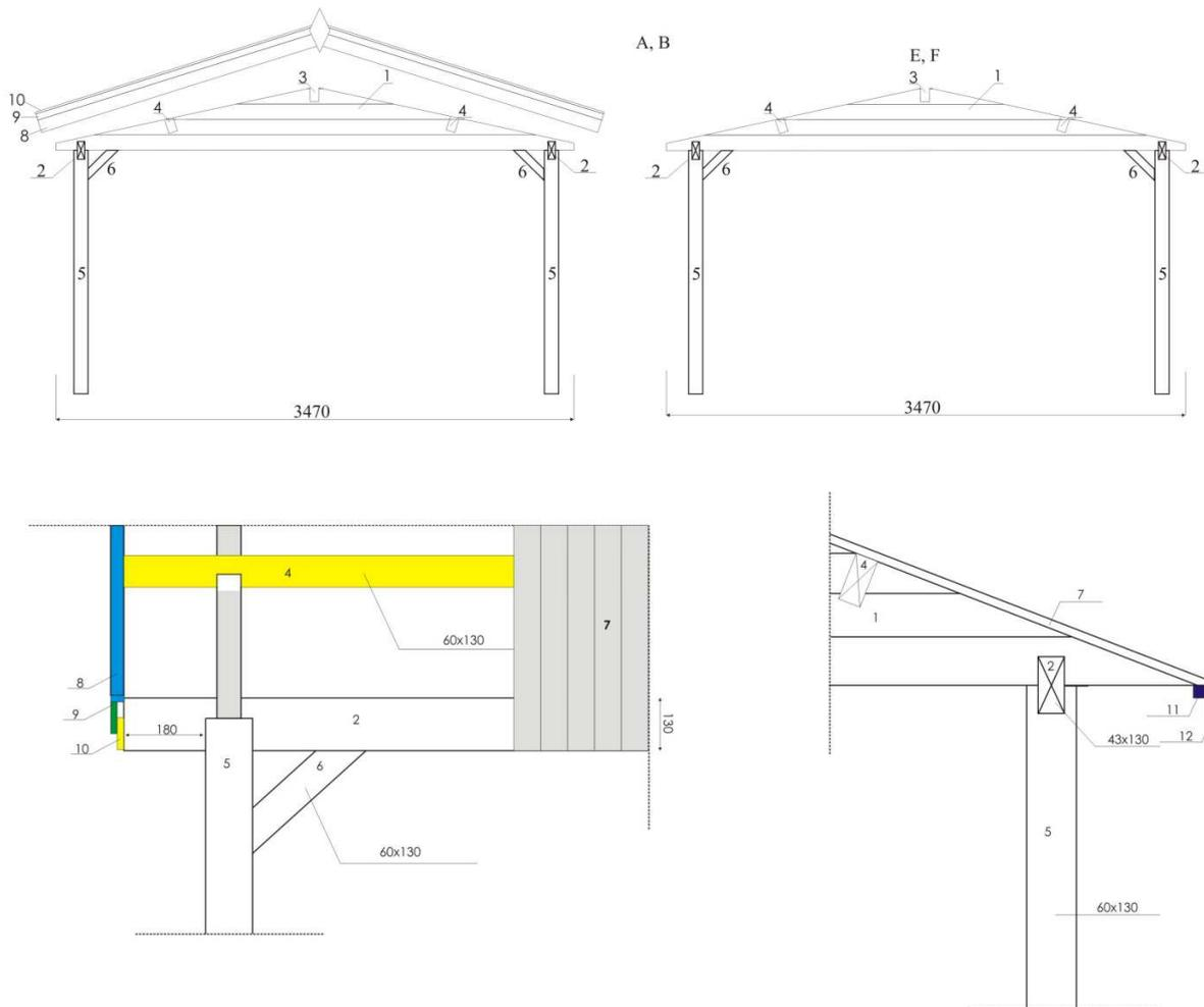
**4.4. Roof-boards:** Attach the roof-boards vertically and screw them into the rafters as shown in the page 3. Make sure the ends of the roof-boards are perfectly parallel to each other. Then fix the roof plank boarder under the roof-boards. The roof-plank must be screwed to the roof plank boarder.
